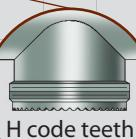
Transitions and adapters are available in a number of configurations, depending on series and system. Versions with H code teeth (shown) for either direct attachment to MIL-DTL-38999 connector adapters, or to additional lengths of conduit, accommodate self-locking coupling nuts for anti-decoupling and easy clocking of backshells and fittings.
