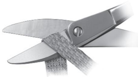
**Note:** When cutting braid, both metal and especially composite, open cutter blades to allow the full 2" cut. Place braid all the way back onto blades as shown.
