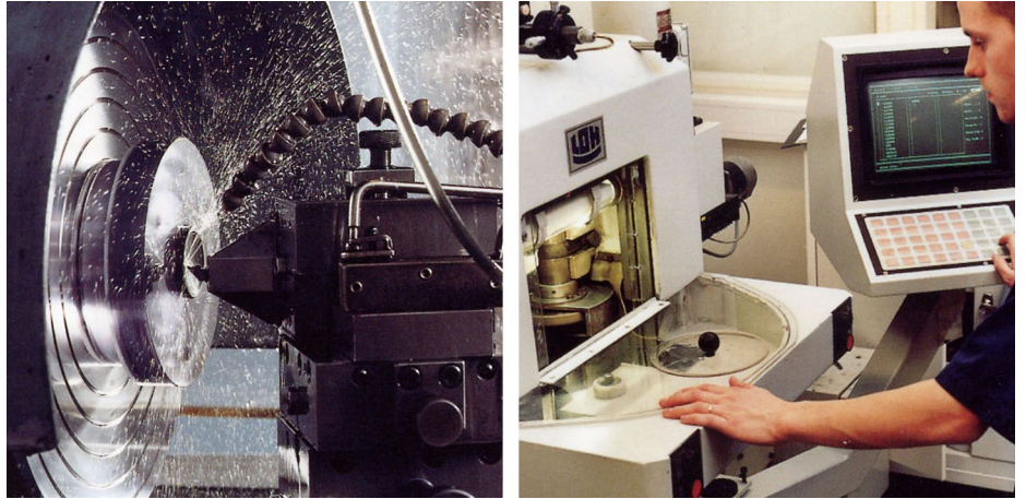
Figure 2.3 LEFT: Diamond turning machine; RIGHT: Lens polishing
