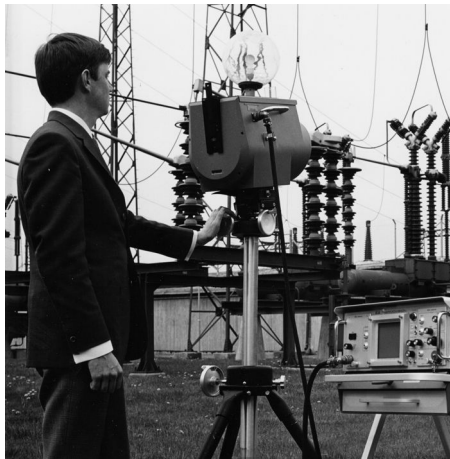
Figure 2.1 1969: Thermovision Model 661. The camera weighed approximately 25 kg (55 lb.), the oscilloscope 20 kg (44 lb.), and the tripod 15 kg (33 lb.). The operator also needed a 220 VAC generator set, and a 10 L (2.6 US gallon) jar with liquid nitrogen. To the left of the oscilloscope the Polaroid attachment (6 kg/13 lb.) can be seen.
