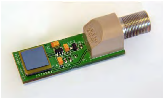
Figure 1: PS25012A3 single channel board carrying a single PS25203 sensor
