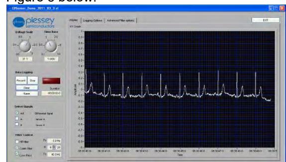
Figure 3: Differential signal from two sensors in contact with the skin showing ECG type characteristics
