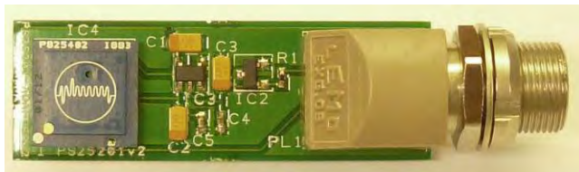
Figure 1: PS25014A2 single channel board carrying a single PS25402 sensor
