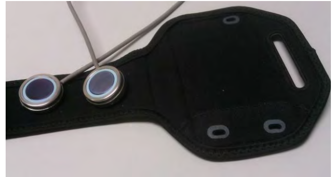
Figure 8 – PS25101 sensors mounted on a commercially available Sports Armband mobile
