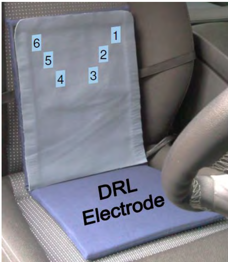
Figure 2 – Showing locations of the 6 sensors and the DRL fabric electrode
