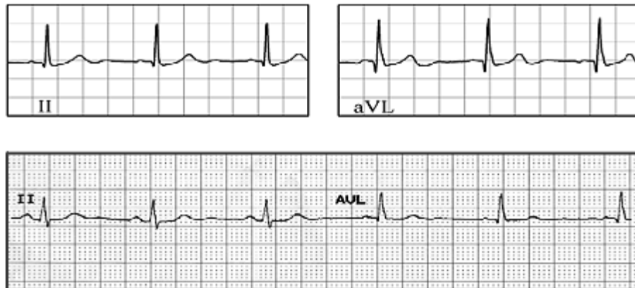
Fig. 8 Comparison of two vectors from a pair of EPIC sensors (top) and two conventional Ag/AgCl electrodes (bottom)
