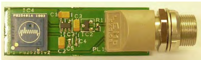
Figure 1: PS25014A1 single channel board carrying a single PS25401A sensor
