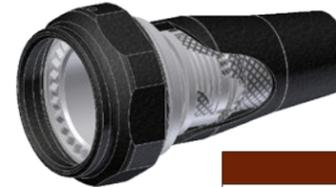
This integrated EMI/RFI shield sock, with its partially recovered shrink-boot and composite connector backshell delivers speed, convenience, and performance. Simply couple in place, terminate the supplied shield to the cable and complete the recovery of the boot.
