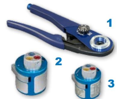
**1** Crimp tool for use with size #20, #16 and #12 power pins. 9.75 inches OAL, 1.25 pounds. Use with M39029/57 and /58 contacts and 809-093 adapters.
