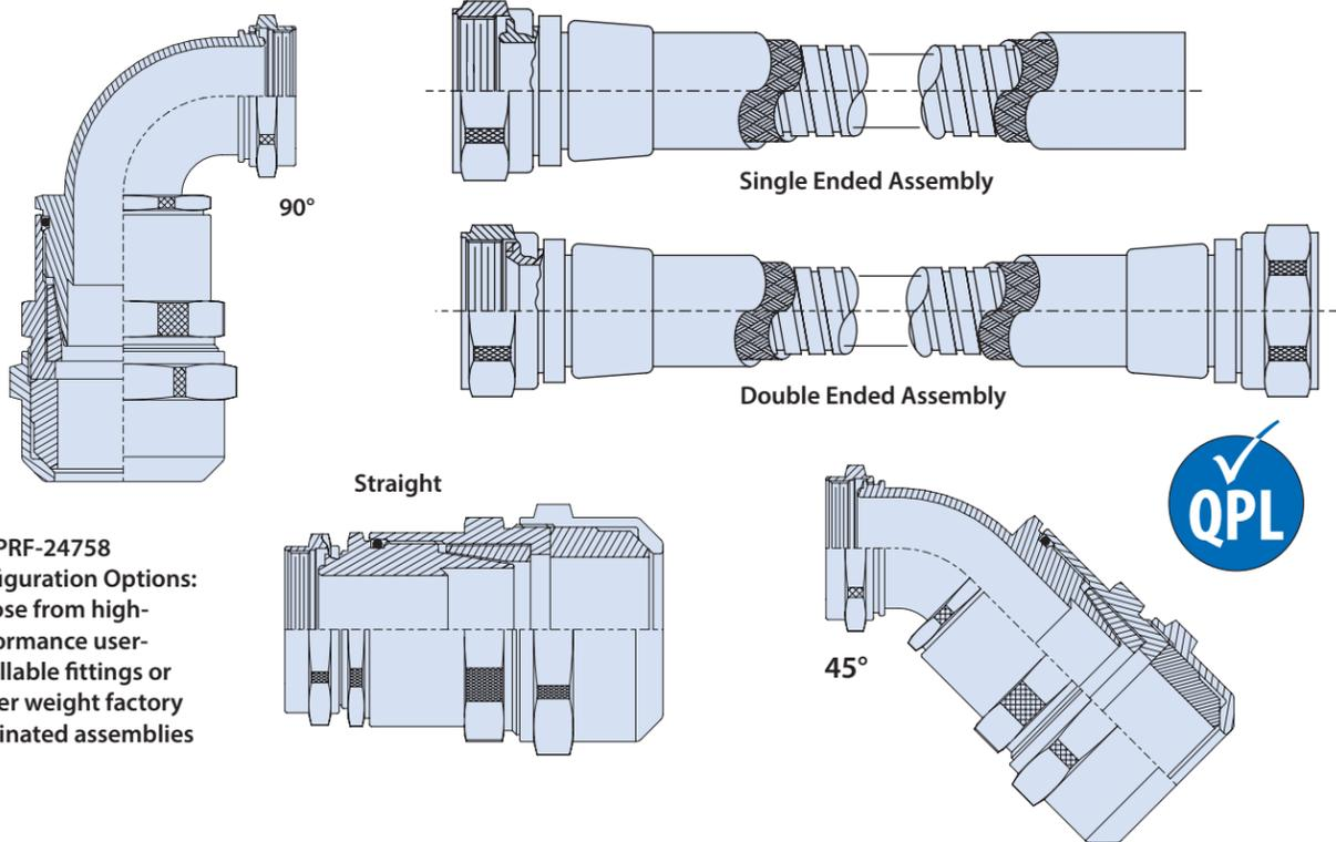
MIL-PRF-24758 Configuration Options: Choose from high-performance user-installable fittings or lighter weight factory terminated assemblies
