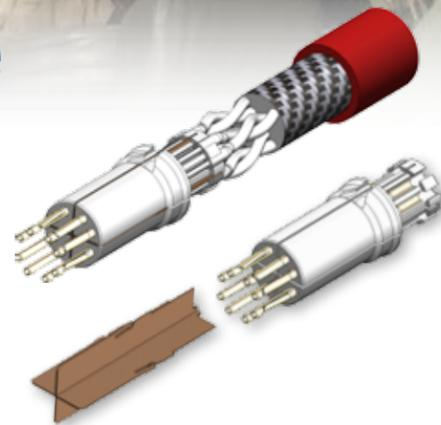
El Ochito™ exploded view: High mating durability, lightweight contact system with 100 Ohm shielded performance. Note wire twist maintained to contact pair to minimize characteristic impedance mismatch. Also, Conductive isolation shield dramatically reduces crosstalk
