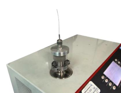
Gas tube helium leak test equipment
