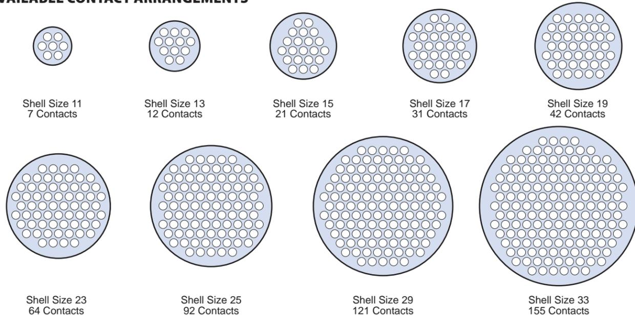
STANDARD PIN CRIMP CONTACT FOR MIL-DTL-28840 CONNECTORS
