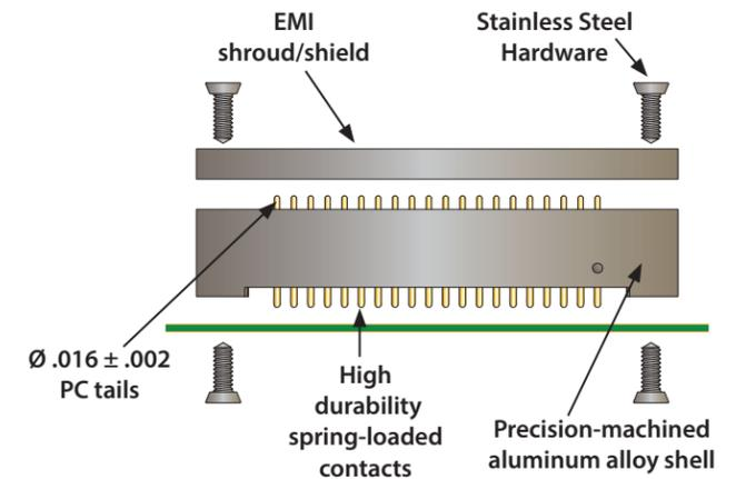
**AlphaLink SL flex jumpers:** Compact interconnect assemblies that combine circuit board technology and cabling into a lightweight, integrated package. These turnkey jumper assemblies reduce system size and weight and are ideally suited for prototype applications and new product development efforts.
